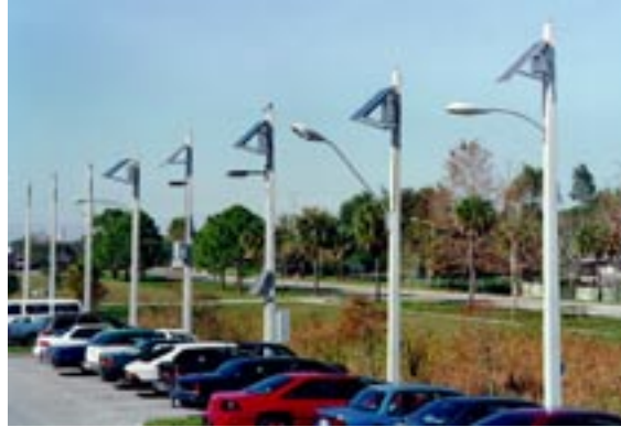
Figure 24. A variety of solar exterior lights undergoing testing at the Florida Solar Energy Center.
