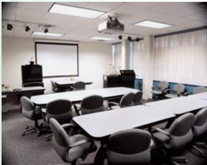
Figure 18. T-bar ceilings, such as the one in this classroom, do not perform well as an air barrier.
