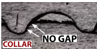
The swaged collar forms over the lock thread, and eliminates the gap.
