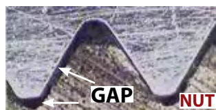
Regular nuts and bolts have gap, which allows for loosening by vibration.
